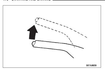
Before leaving the vehicle, make sure that the parking brake is set. To set the parking brake, pull up firmly on the lever. Also place the gear selector in the Park position (automatic transaxle) or Reverse (manual transaxle). To release the parking brake, apply the brake pedal and pull up on the parking brake lever. Push the release button and lower the lever fully.
